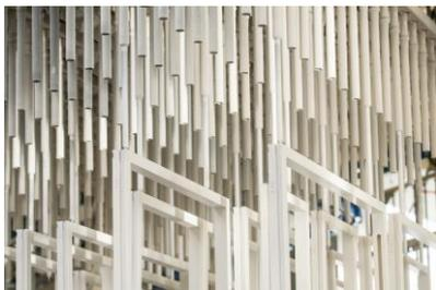
■ The operator hangs the parts on the conveyor
